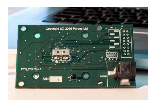
The Broadcom® ezPyro™ application-specific evaluation kits demonstrate the capabilities of Broadcom's innovative ezPyro digital SMD infrared sensors. The evaluation kits consist of a main board with up to four ezPyro sensors and an attached controller board based on an ARM Cortex-M4 microcontroller. There are specific kits for gas, flame, motion, and gesture sensing, as well as a generic kit that allows various ezPyro sensors to be plugged into a backplane board.
