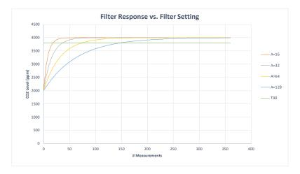
The graph above shows the effect of the filter on response times. Increasing the filter setting increases the measurement output response time.  $T_{90}$  is the time to 90% of reading. The ExplorIR®-M takes 2 readings per second.
