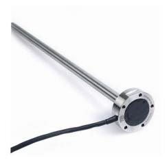
Capacitive level sensing technology has no moving parts. The sensor measures the relative permittivity of the liquid and compares that to air. By knowing the relative permittivity values at two states, full of liquid and "full" of air, the sensor can calculate the level in real time.
