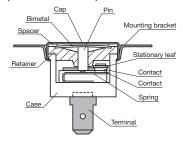
By forming a bimetal strip into a dome shape (hemispherical, dished shape) to acquire snap action, the disk type protector is characterized by its simplicity of construction. The simple design facilitates volume production and, because of its low cost, account for 80% of the entire bimetallic thermal protector market in the world.
